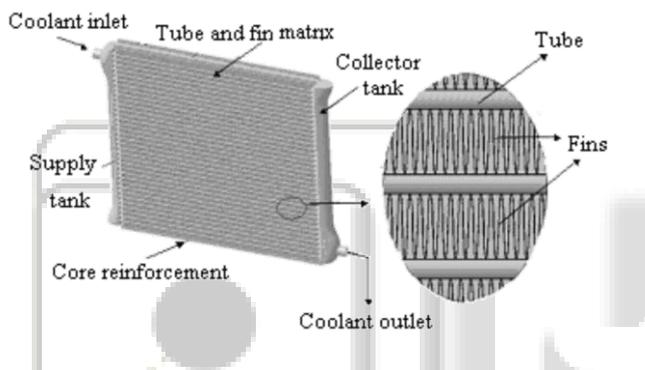
Fig. 3: Assembled CATIA model of the radiator
