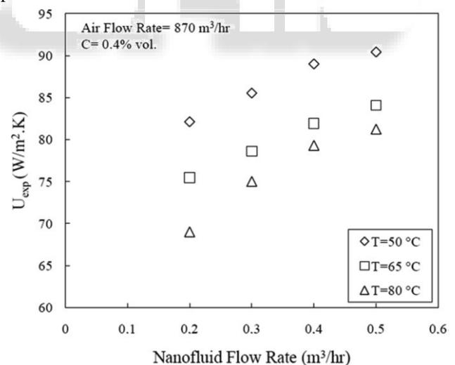
Fig. 1: Effect of nanofluid volumetric flow rate on the overall heat transfer coefficient of CuO/water nanofluid in the radiator.
