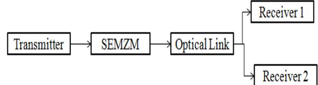
Fig. 4: Block Diagram External modulation using SEMZM
