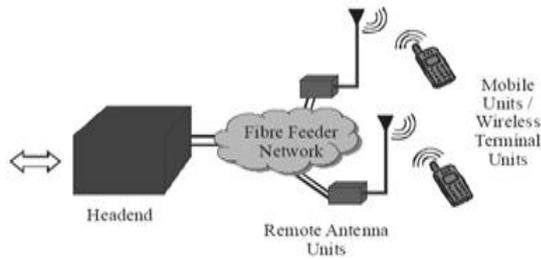
Fig. 2: Block diagram Radio over Fiber System
