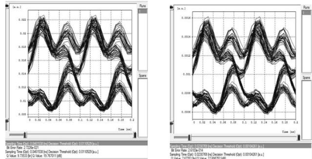
Fig. 7: Eye diagram of External Modulation Using DEMZM obtained from (a) EDFA (b) SOA at 20 Km
