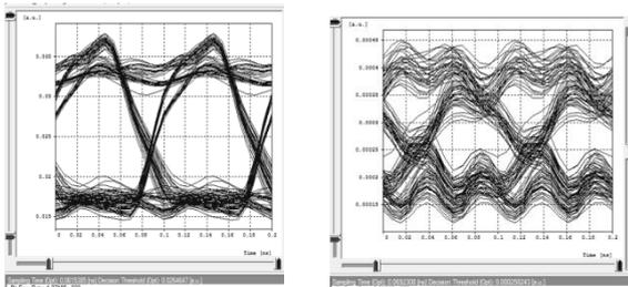
Fig. 15: Eye diagram of External Modulation Using SEMZM obtained from (a)EDFA (b) SOA at 30 Km
