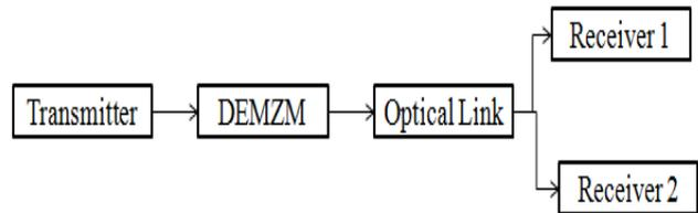
Fig. 3: Block Diagram External modulation using DEMZM
