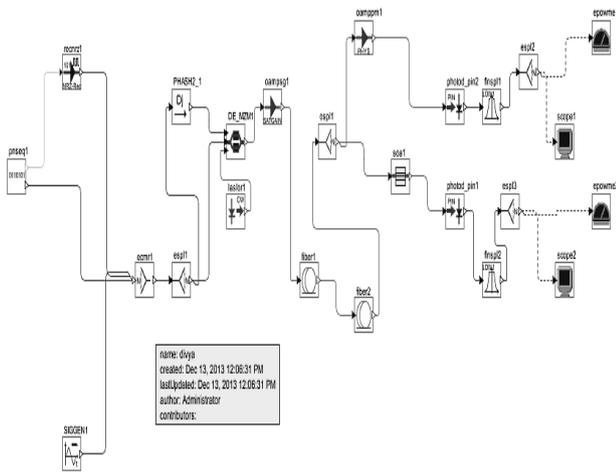
Fig. 5: Simulation setup of External modulation using DEMZM
