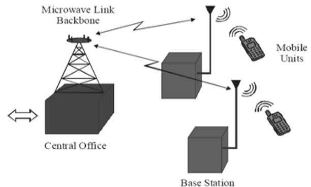
Fig. 1: Components of a Narrowband Wireless Access Network
