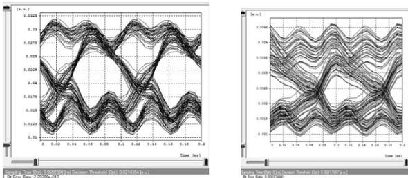
Fig. 16: Eye diagram of External Modulation Using SEMZM obtained from (a)EDFA (b)SOA at 40 Km
