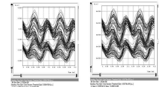
Fig. 9: Eye diagram of External Modulation Using DEMZM obtained from (a) EDFA (b) SOA at 40 Km
