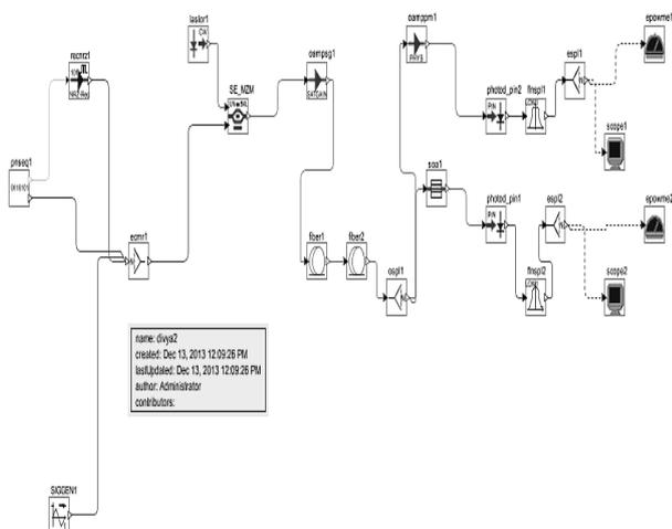
Fig. 6: Simulation setup of External modulation using SEMZM
