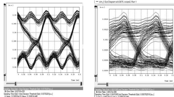
Fig. 14: Eye diagram of External Modulation Using SEMZM obtained from (a)EDFA (b) SOA at 20 Km
