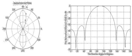
Fig. 5: optimized Radiation pattern using Genetic Algorithm having side lobe level
