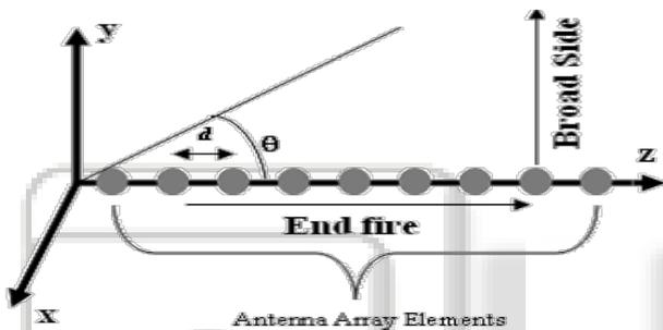
Fig. 2: Linear antenna array
