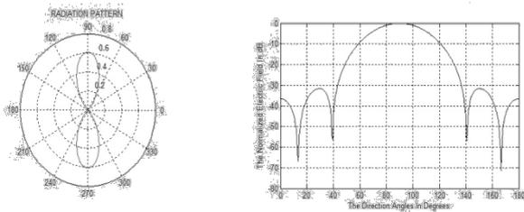
Fig. 6: optimized Radiation pattern using Big Bang Crunch having side lobe level
