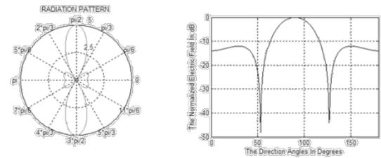
Fig. 3:Un-optimized Radiation pattern.
