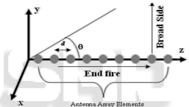
Fig. 1: Antenna Array
