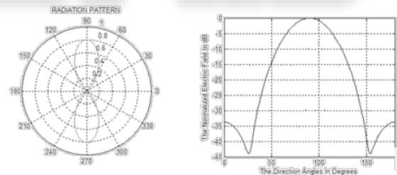
Fig. 5: Optimized Radiation pattern using CHAOTIC Optimization Algorithm.
