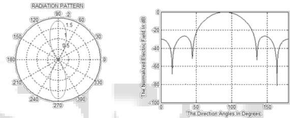
Fig. 4: Optimized Radiation pattern using Genetic Algorithm
