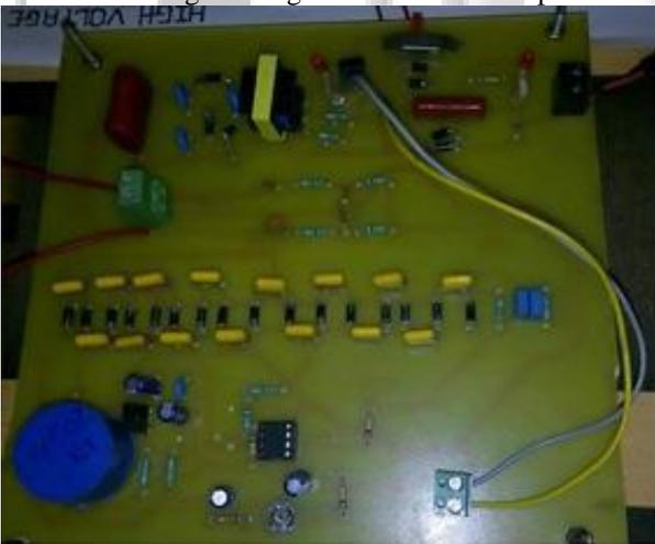
Fig. 6: Prototype setup of Cockcroft-Walton multiplier circuit
