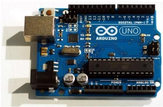
Fig. 1: ARDUINO ATMEGA 328 Microcontroller
