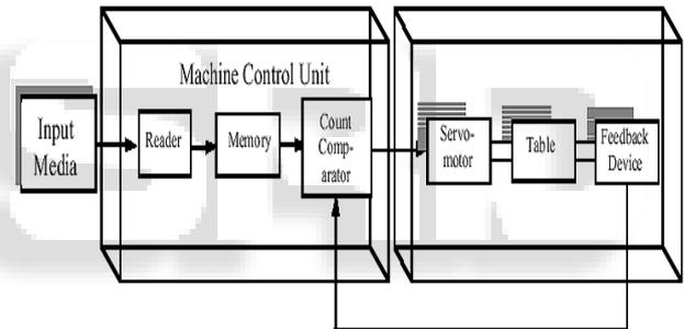
Fig. 2: Major components of a numerical control machine tool
