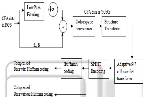
Fig. 5: Proposed Scheme of structure of image compression algorithm flow
