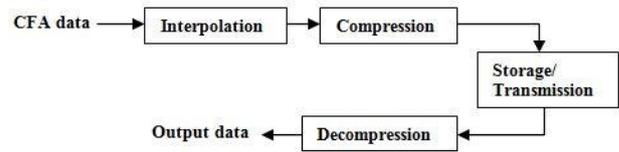
Fig. 2(a): Arrangement of Interpolation before compression
