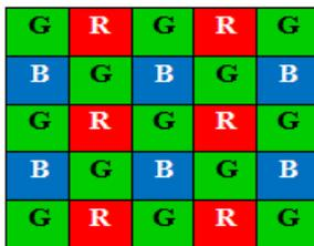
Fig. 1: Arrangement of Bayer Pattern CFA
