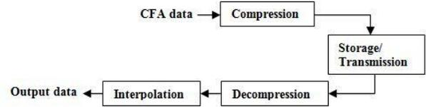
Fig. 2(b): Arrangement of Compression before interpolation
