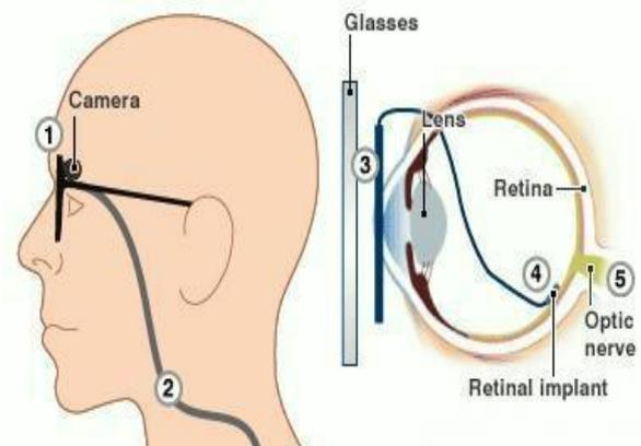
Fig. 1: Bionic eye system
