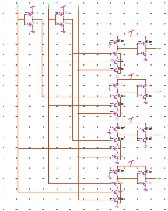
Fig. 10: Schematic of Pseudo logic multiplexer on tanner tool
