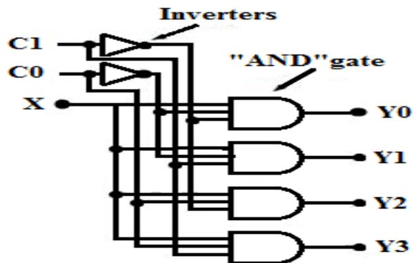
Fig. 2: Conventional CMOS 1:4 De-multiplexer
