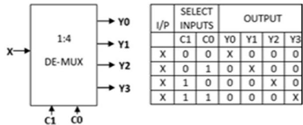
Fig. 1: De-multiplexer and its truth table
