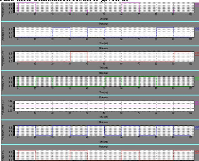
Fig. 9: Simulation result of Transmission gate De-mux
