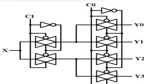
Fig. 4: 4 De-multiplexer circuit using Transmission gate
