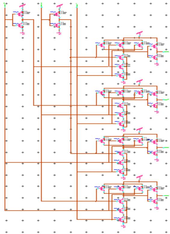
Fig. 6: Schematic of CMOS 1:4 De-multiplexer on tanner tool
