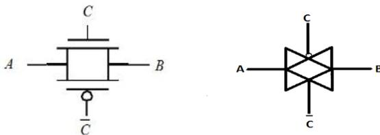
Fig. 3: Schematic and circuit symbol of Transmission gate
