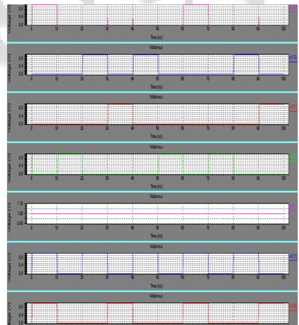
Fig. 11: Simulation result of Pseudo logic based 1:4 De-mux
