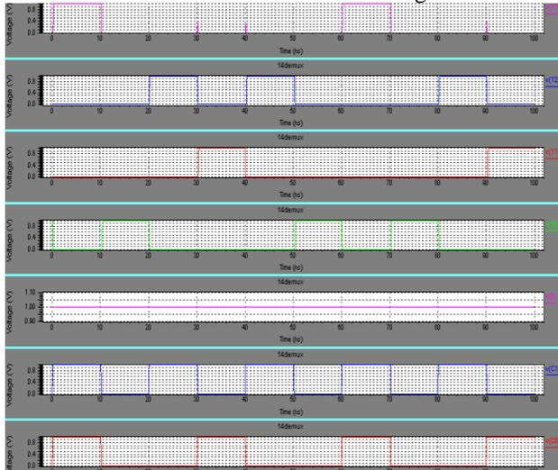
Fig. 7: Simulation result of CMOS 1:4 De-multiplexer
