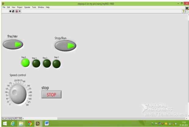
Fig. 6: Front panel of LabVIEW Stepper control.vi
