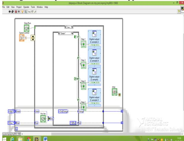
Fig. 7: Block diagram off LabVIEW Stepper control.vi
