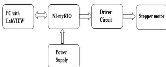
Fig. 1: Schematic block diagram of stepper motor control loop
