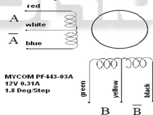
Fig. 2: Schematic diagram of unipolar stepper motor winding
