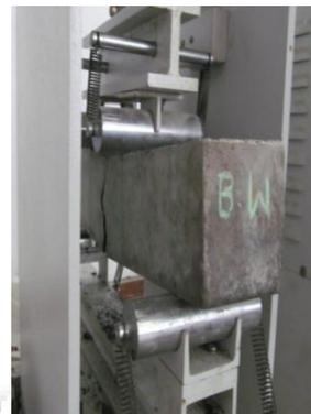
Fig 7:Flexural Test
