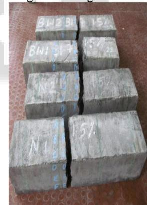
Fig. 10: Beams in Flexure
