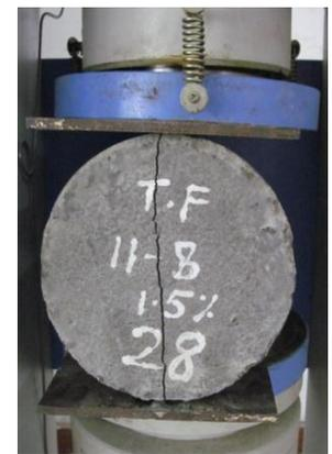
Fig. 6: Split Tensile Test
