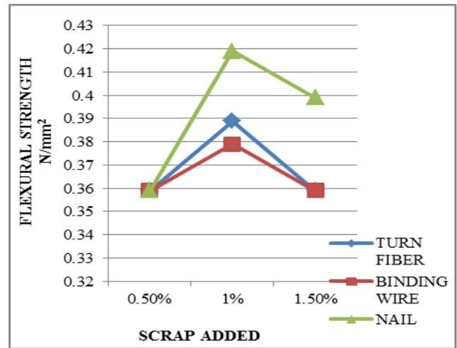
Fig. 16: 28 Day Flexural Test
