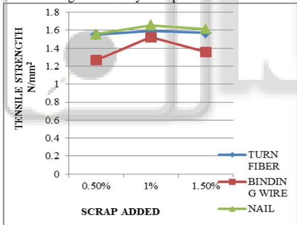
Fig. 14: 7 Day Split Tensile Test
