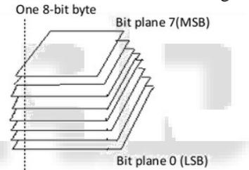
Fig. 14: Bit Plane representation of an 8 bit image
