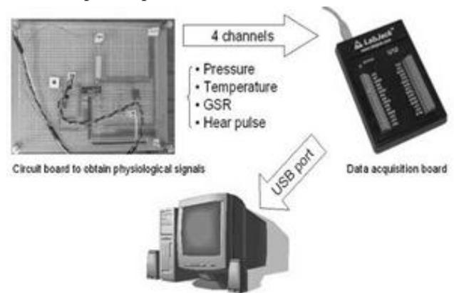
Fig. 4.2: System Configuration for Emotional Mouse
