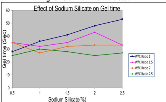
Fig. 9: Sodium Silicate v/s Gel time
