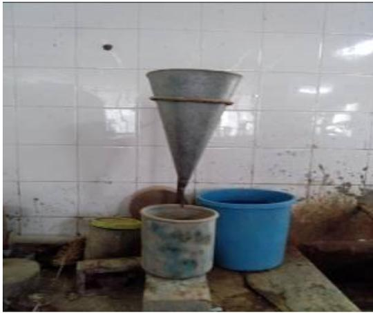
Fig. 2: Set up for Marsh Cone Test
