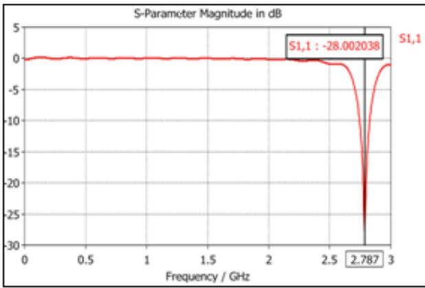
Fig. 2: Return loss S1, 1 of Rectangular Microstrip Patch Antenna
