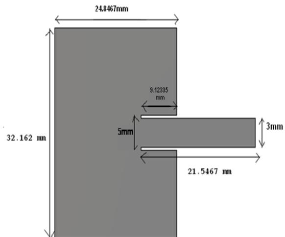
Fig. 1: Rectangular patch antenna at 2.787 GHz.
