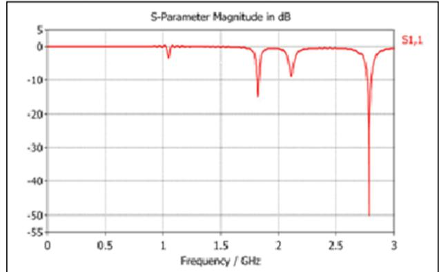
Fig. 5: Simulation of Return Loss S1, 1 RMPA with proposed metamaterial structure
