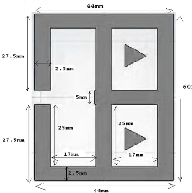
Fig. 3: structure of the proposed antenna dimensional view
