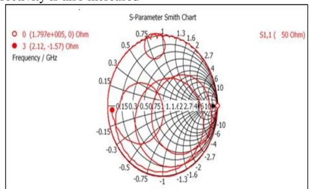
Fig. 6: Smith chart of PMPA loaded with metamaterial.
