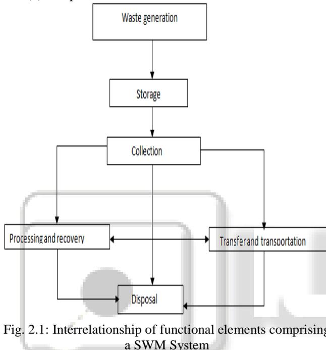
Fig. 2.1: Interrelationship of functional elements comprising a SWM System
