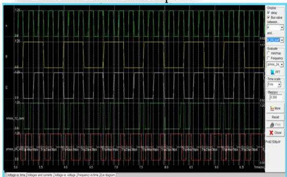
Fig. 6: Voltage versus time waveform for sum and carry logic
