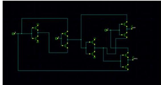
Fig. 7: Circuit design for sum and carry logic of full adder using 10 transistors
