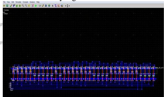
Fig. 5: Layout of full adder in MICROWIND
