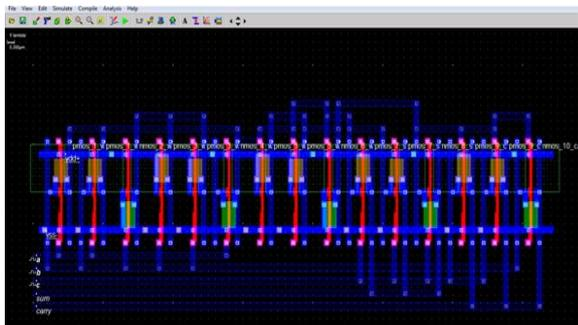
Fig. 9: Layout Design in MICROWIND
