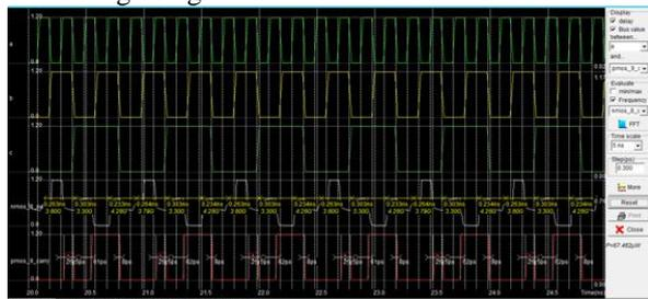
Fig. 10: Voltage versus time waveform for sum and carry logic
