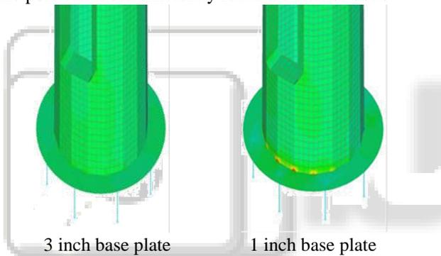
Fig. 2: Comparison of stresses at pole-to-base plate connection for 1 inch and 3 inch base plates
