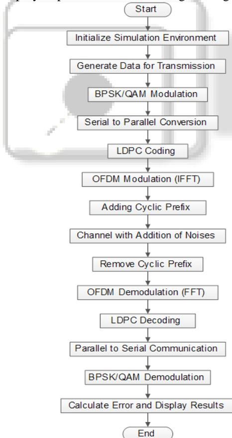
Fig. 2: Flow chart of the simulation algorithm of proposed shallow water communication system
