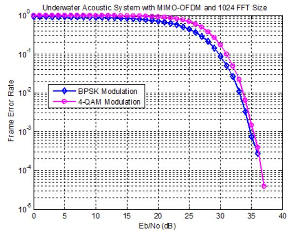
Fig. 6: FER vs SNR curve of shallow water communication with MIMO-OFDM System using 1024-Bit FFT Size
