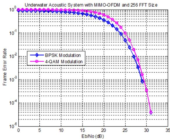
Fig. 4: FER vs SNR curve of shallow water communication with MIMO-OFDM System using 256-Bit FFT Size
