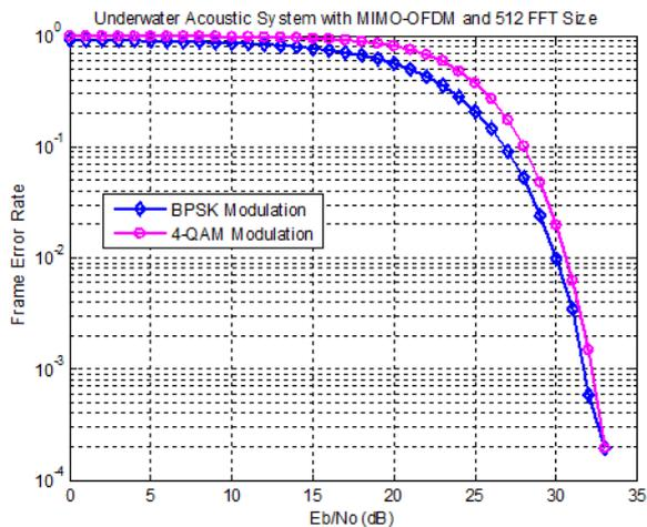
Fig. 5: FER vs SNR curve of shallow water communication with MIMO-OFDM System using 512-Bit FFT Size
