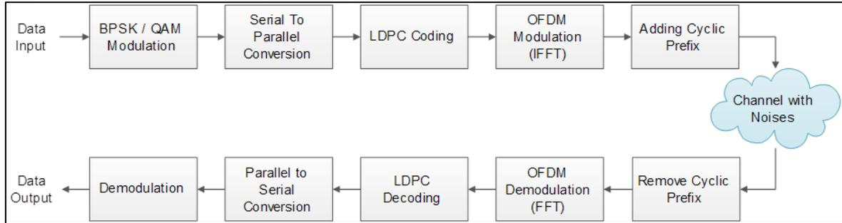
Fig. 1: Block diagram of the proposed shallow water communication system
