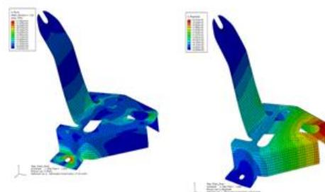
B. Base Model 1: Thickness = 2mm
