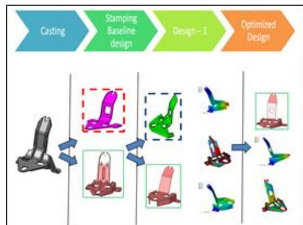
Fig 3: Shows the tree diagram for stages of a VSA Bracket
