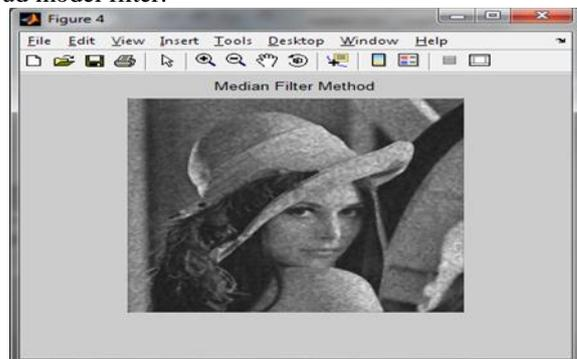
Fig. 8: Restored Image using the median filter
