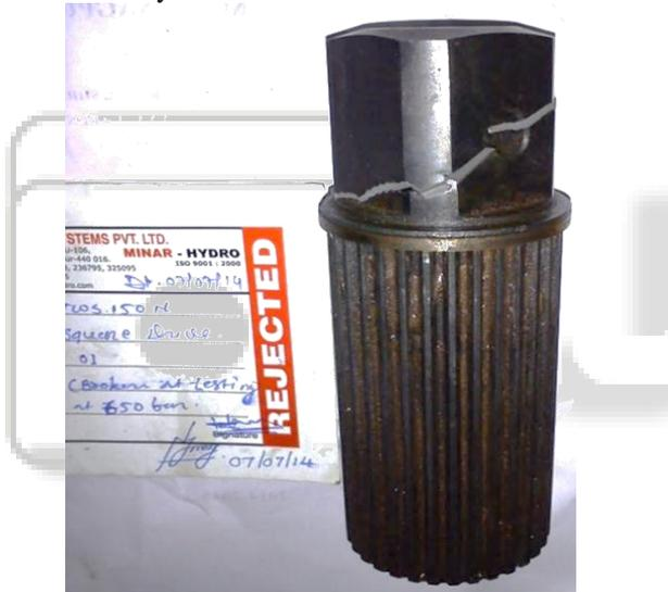
Fig. 3: Failure component (DMR 1700 steel) of hydraulic torque wrench by twisting force acting on it.
