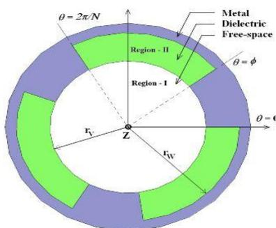
Fig. 2: Dielectric and vane-loaded circular waveguide
