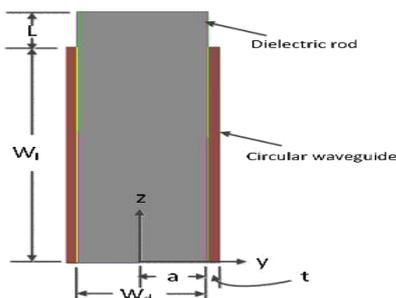
Fig. 1: Circular waveguide loaded with dielectric rod
