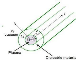
Fig. 3: Geometry of dielectric tube filled with plasma
