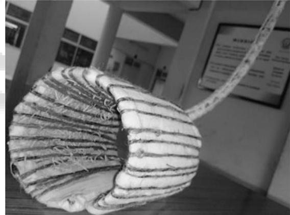
Fig. 2: Structure of capillary jacket and capillary tube
