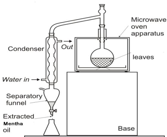
Fig. 1: Microwave extraction apparatus.
