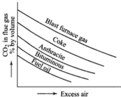
Fig. 1: Variation in flue gas with fuels and excess air
