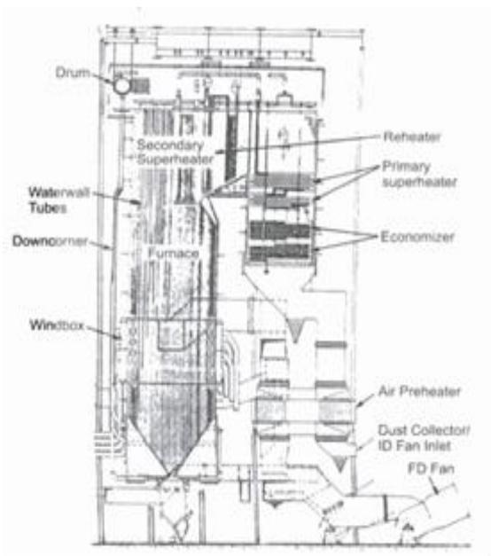
Fig. 4: General Arrangement of Pulverized Coal Fire Boiler
