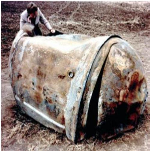
Fig. 2: Two large fragments of a Delta second stage
