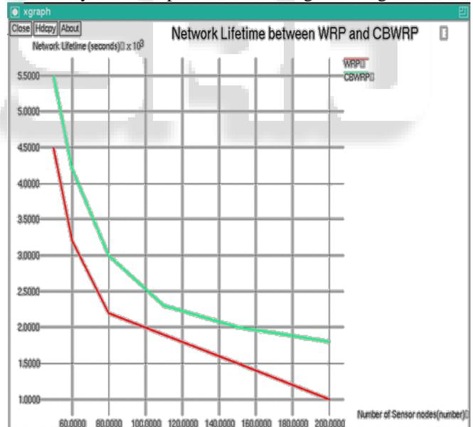
Fig. 3: Network Lifetime between WRP and CBWRP.
