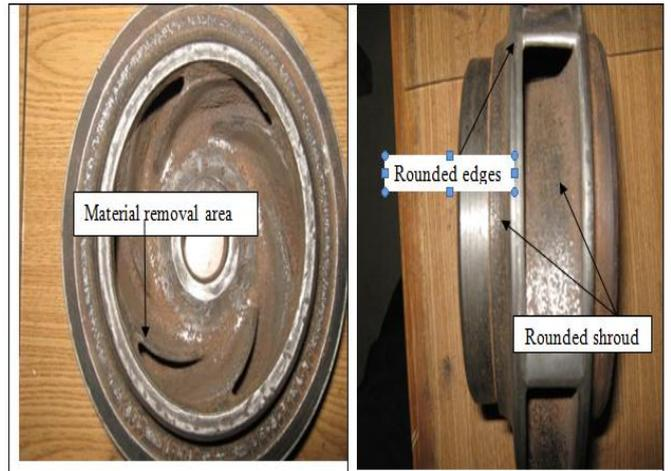
Fig. 6: PAT Impeller with modification
