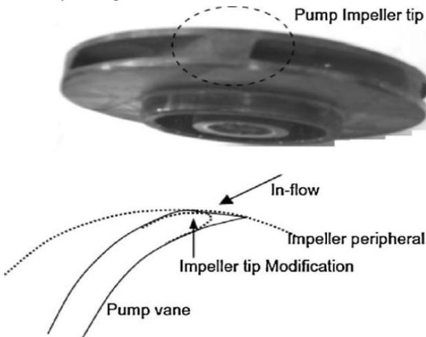
Fig. 5: Modified Impeller
