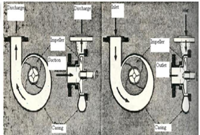
**Pump in pumping and turbine mode**
