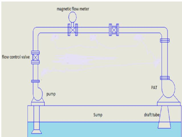
Fig. 2: Experimental Test-Rig and Instrumentation
