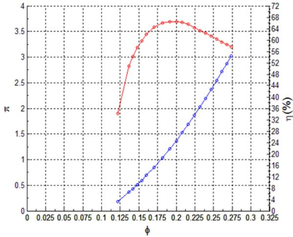
Fig. 3: Power number and efficiency vs flow number characteristic of PAT without modified impeller
