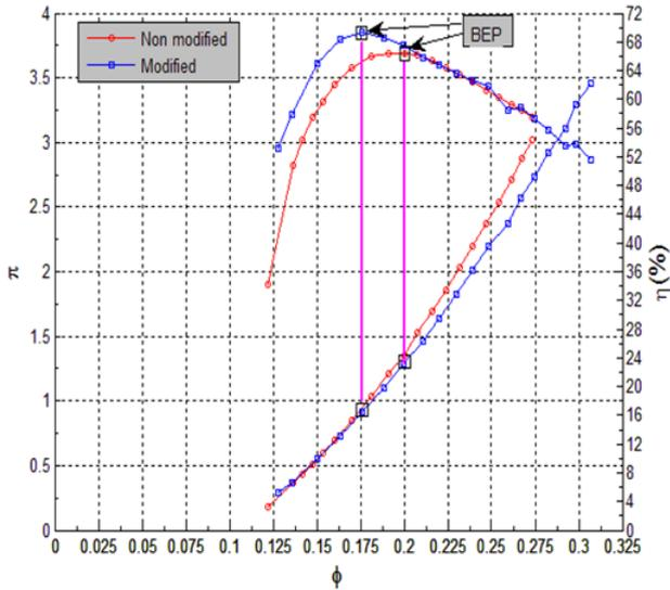
Fig. 9: Comparison of power number and efficiency of PAT with and without modified impeller
