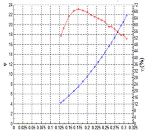
Fig. 8: Head number and efficiency Vs flow number characteristic of PAT with modified impeller
