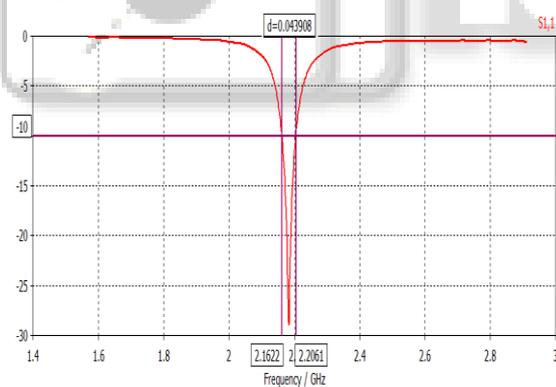
Fig. 7: Bandwidth of designed microstrip patch antenna
