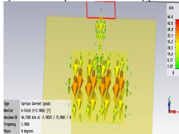
Fig. 11: Surface current of designed microstrip patch antenna
