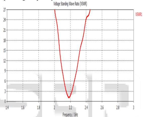
Fig. 10: VSWR of designed microstrip patch antenna
