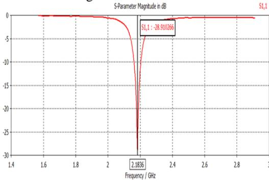
Fig. 6: Return loss of the designed microstrip patch antenna. The center frequency is selected as the one at which the return loss is minimum. The bandwidth can be calculated from the return loss (RL) plot. The bandwidth of the antenna can be said to be those range of frequencies over which the RL is greater than -9.5 dB (-9.5 dB corresponds to a VSWR of 2 which is an acceptable figure). Using the optimum feed depth is found to be at  $y_0 = 11.8333$ mm where a RL of -28.910266 dB is obtained.
