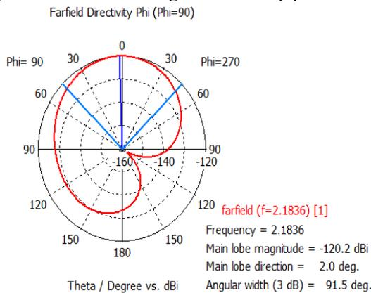
Fig. 8: Elevation pattern for  $\phi = 90$  degrees
