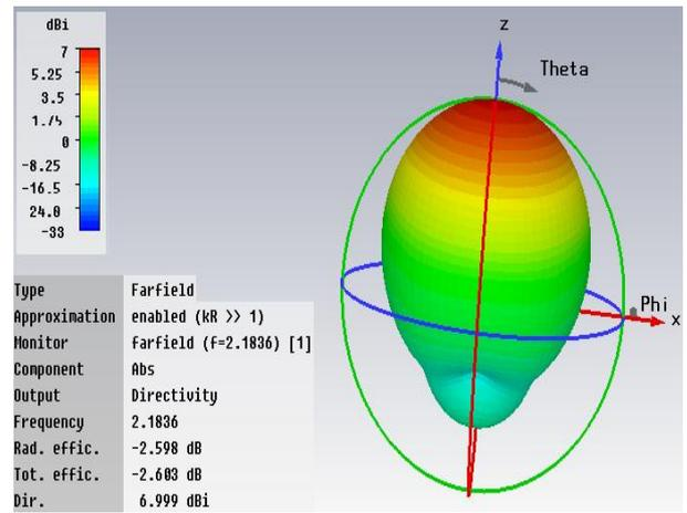
Fig. 9: 3 D radiation pattern of designed antenna
