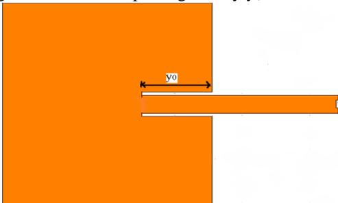
Fig 5: An inset feed microstrip patch antenna
