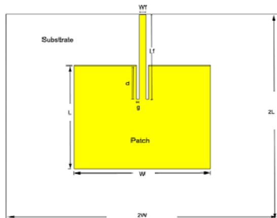
Fig. 4: Dimensions of an inset feed microstrip patch antenna
