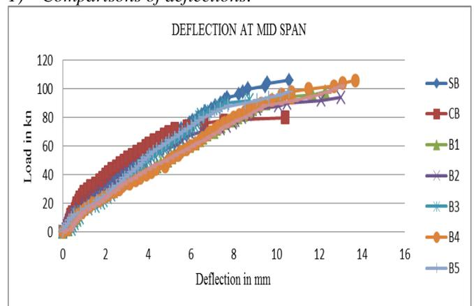
Fig. 3: Load-deflection relationship for all beams at mid span
