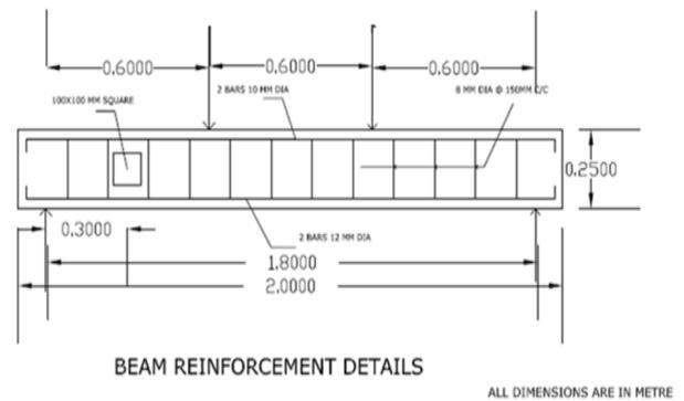
Fig. 1: Dimension of beam with square opening in shear zone
