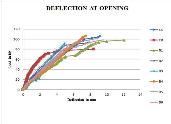
Fig. 4: Load-deflection relationship for all beams opening
