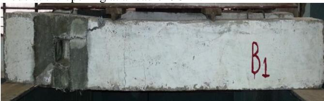
Fig. 5: cracking pattern for the strengthened beam B1 with GFRP around the opening
