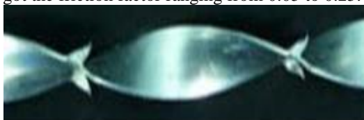
Fig. 3: Delta-Winglet Twisted Tape
