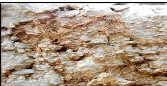
Fig. 6: Recron-3s fiber in concrete
