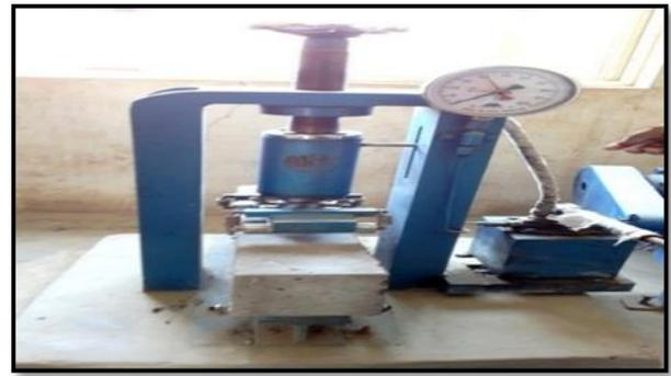
Fig. 9: Testing of Flexural Strength of concrete Beam
