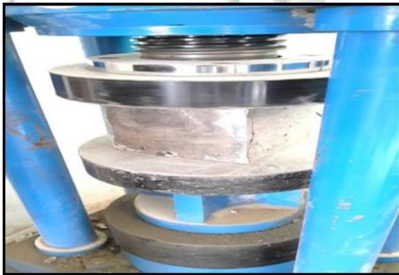
Fig. 8: Compression Test on Recron-3S Material mixing cube
