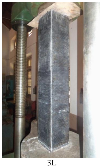
Fig. 4.8: Failure Pattern of CFRP Strengthened Column with Different Layers.
