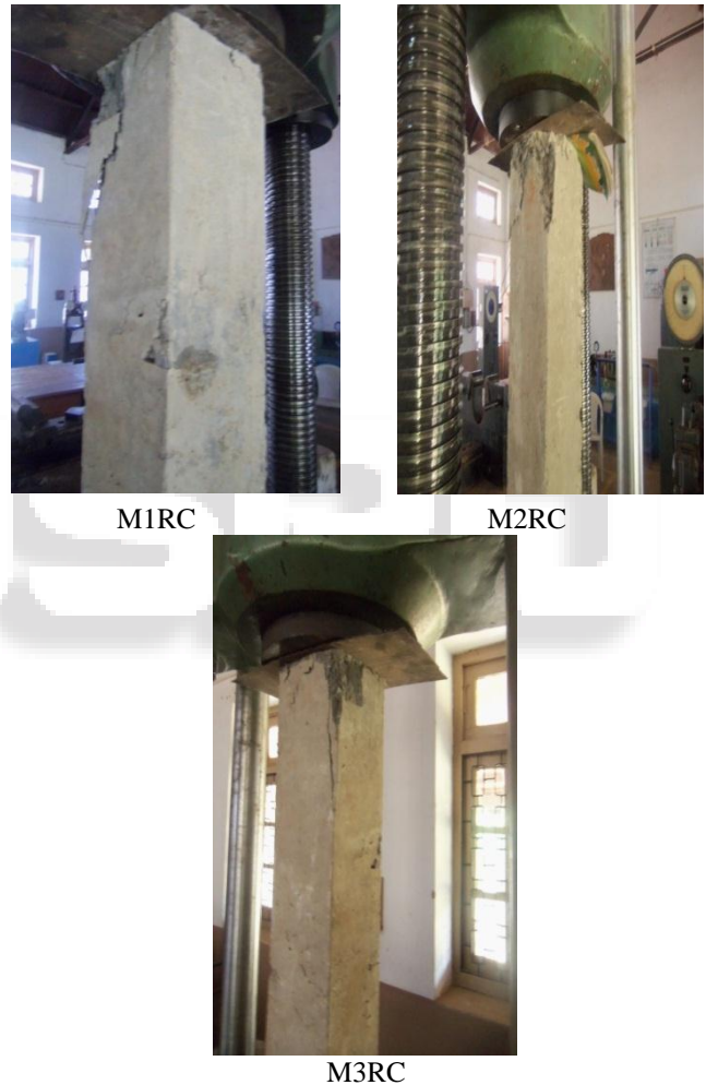
Fig. 4.4: Failure Pattern of RC Column with Different Grade
