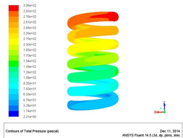
Fig. 6: Total pressure PCD 50mm
