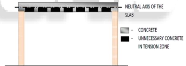
Fig. 1: Unwanted portion of concrete below the neutral axis
