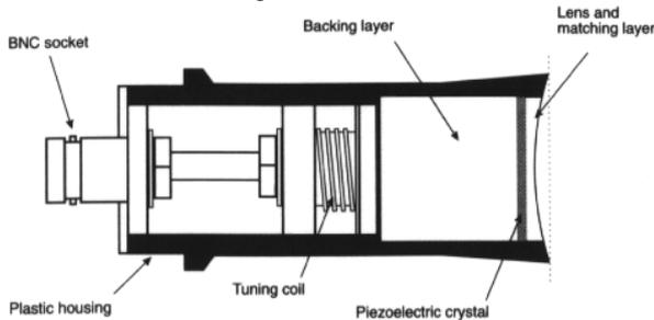
Fig. 8: single element Transducer
