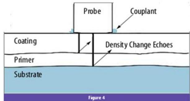
Fig. 4: layers of test material with ultrasonic probe
