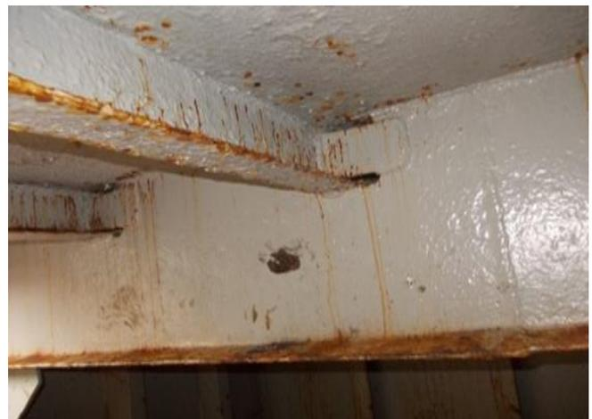
Fig. 5: internal surface of ship hull structure after 5year<sup>[3]</sup>
