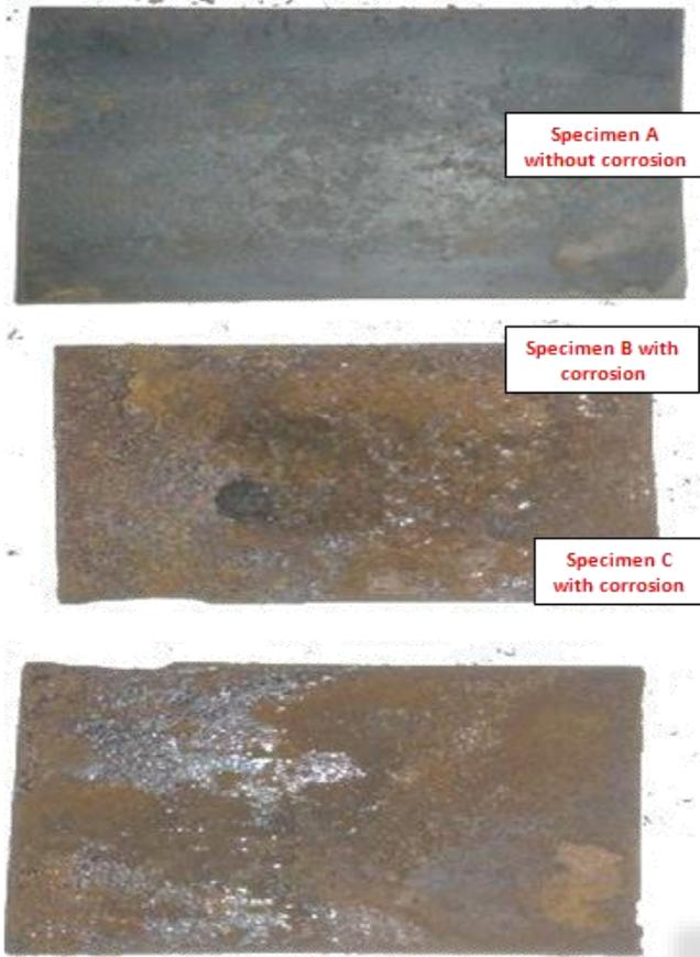
Fig. 11: corrode metal plate after 6 month under corrosion condition
