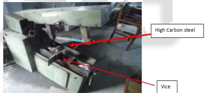
Fig. 6: power hack saw used for cutting purpose
