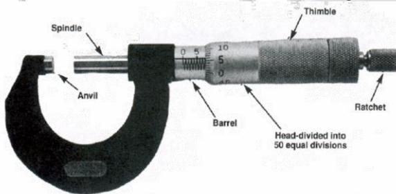
Fig. 9: Micrometer caliper
