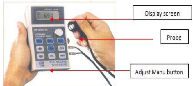
Fig. 7: Ultrasonic thickness gauge
