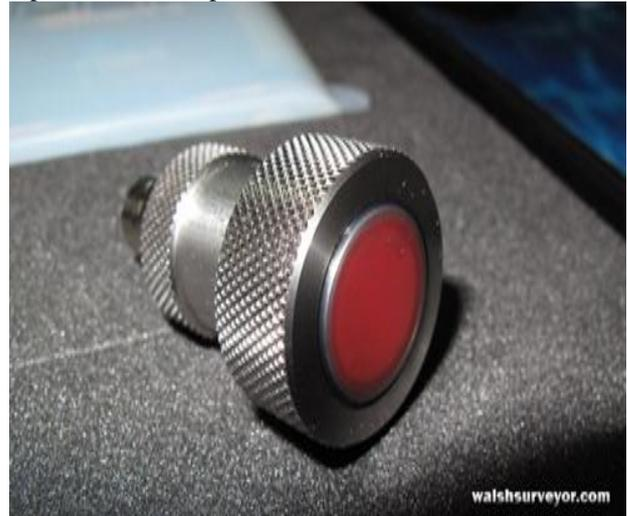
Fig. 6: ultrasonic thickness measuring equipment probe
