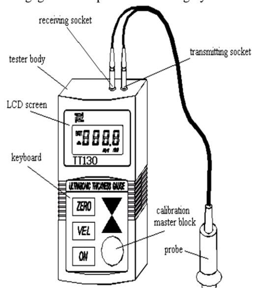
Fig. 1: ultrasonic testing machine <sup>[12]</sup>
