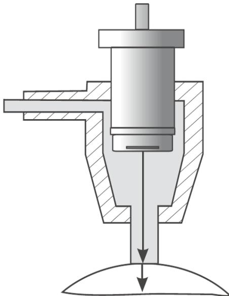
Fig. 2: principle of ultrasonic testing machine<sup>[12]</sup>
