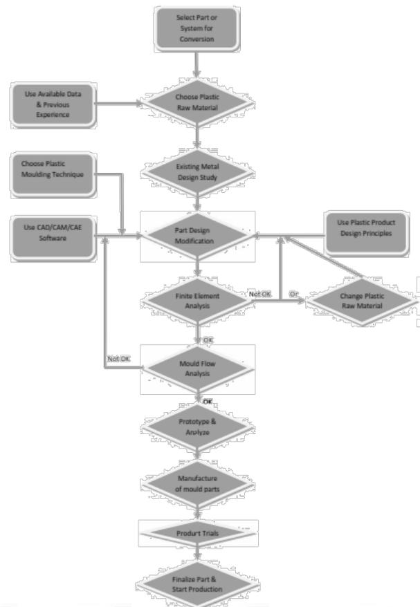
Fig. 1: A Generalized systems approach for metal to plastic conversion
