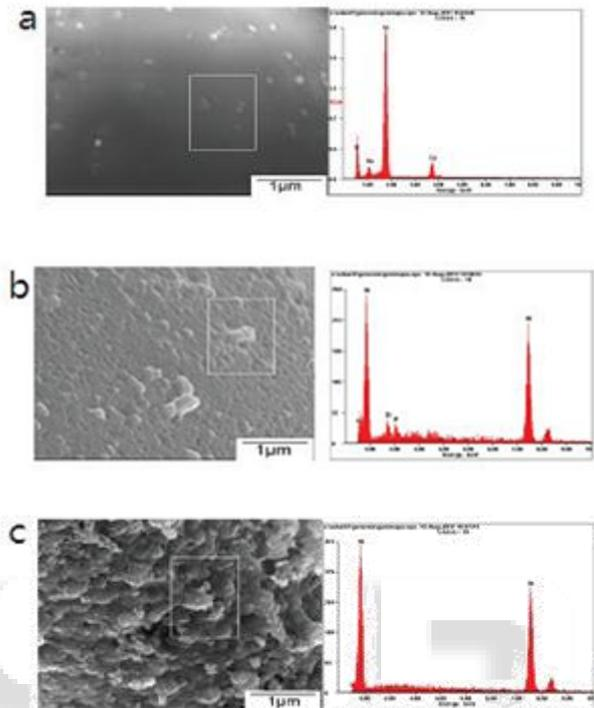
Fig. 4: SEM images and EDS of GBs/Ni-plated GBs/ Ni-plated GBs with heat treatment (a) Before plating; (b) After plating (c) The coating with heat treatment
