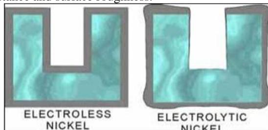
Fig. 1: Comparison between electroless and electroplating surfaces
