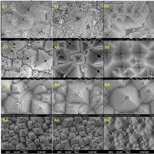
Fig. 5: SEM images (top view) showing variation in surface morphology of electroless nickel deposition due to effect of light
