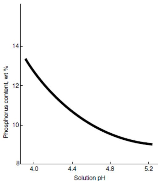
Fig. 3: Effect of pH on phosphorous content.
