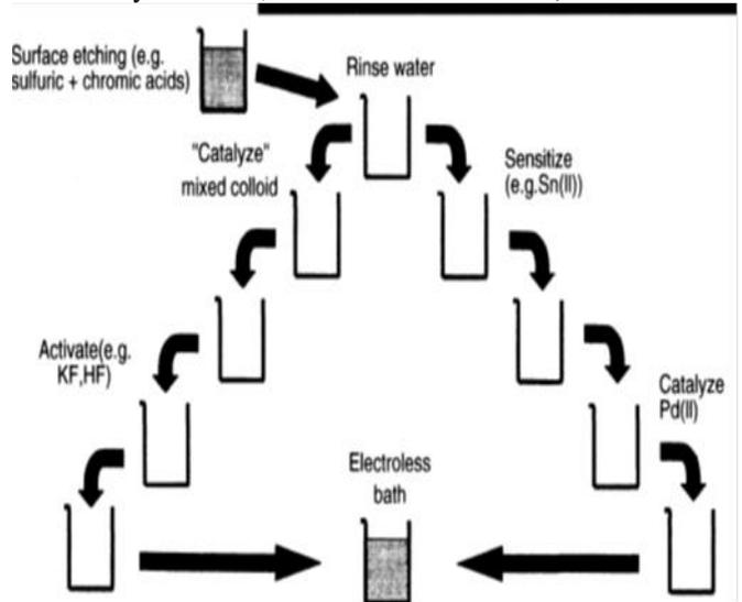
Fig. 2: Schematic representation of the electroless deposition process.
