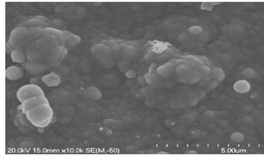
Fig. 6: The surface morphologies of original PerFactory™ model surface, and surface after electroless nickel plating
