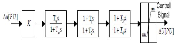
Fig. 4.1: Auxiliary SSR damping controller
