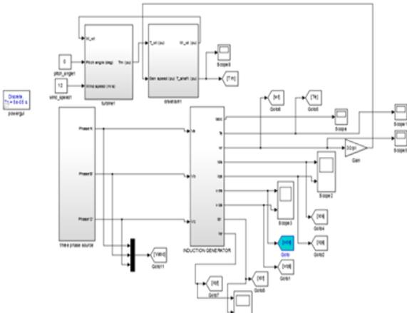
Fig. 2.5: Simulink model of induction generator with turbine and drive train
