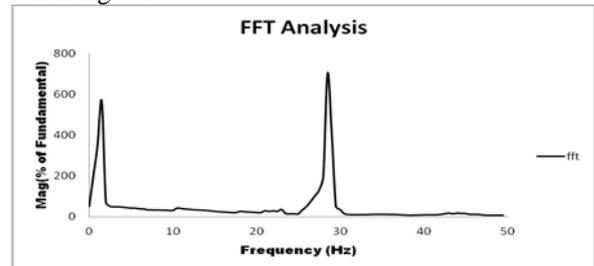
Fig. 3.13: FFT analysis of generator rotor speed
