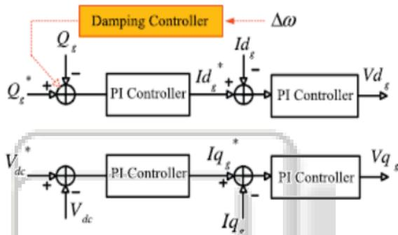
Fig. 2.3: The control structure of the DFIG grid-side converter
