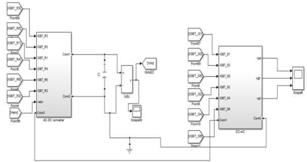
Fig. 2.6: Back-to-back PWM converter
