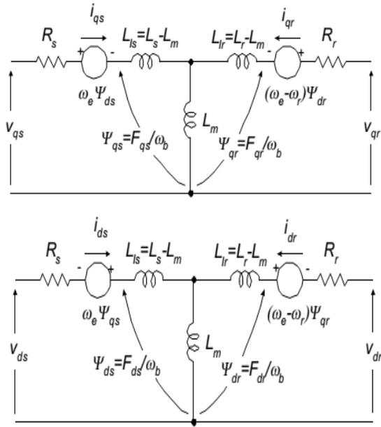
Fig. 2.4: Dynamic or d-q equivalent circuit of induction machine
