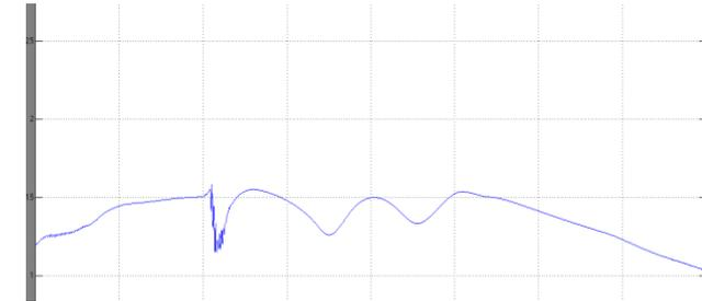
Fig. 4.2: Waveform of generator rotor speed when conventional damping controller is used
