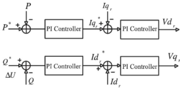
Fig. 2.2: The control structure of the DFIG rotor-side converter
