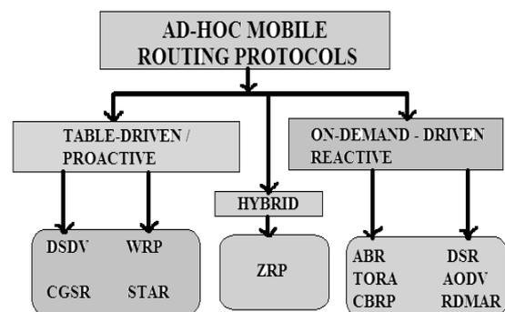
Fig. 2: Ad Hoc mobile routing protocols
