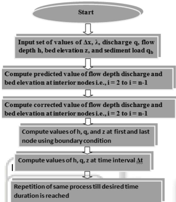
Fig. 4: Programming algorithm
