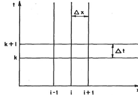
Fig. 3: Finite difference grid
