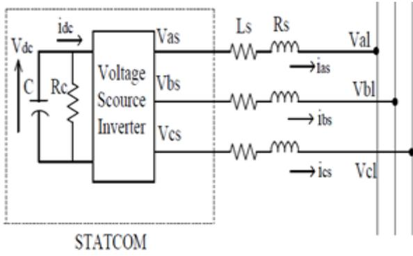
Fig. 2: Equivalent circuit of STATECOM
