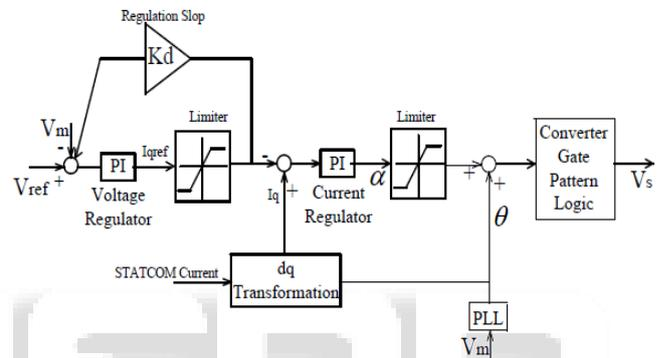
Fig. 3: STATECOM PI control block diagram
