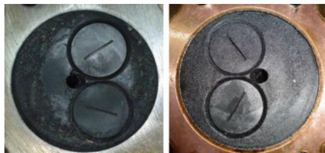
Fig. 2.7: Carbon Deposits On The Cylinder Head Of The Engine (A) Using EGR (B) Without EGR
