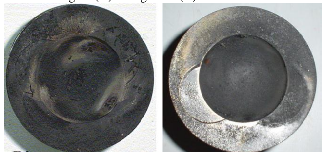
Fig. 2.8: Carbon Deposits On The Piston Crown Of The Engine (A) Using EGR (B) Without EGR
