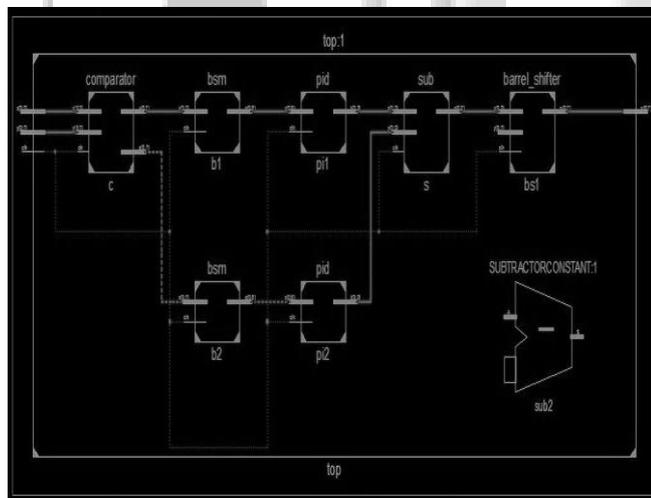
Fig.6 RTL schematic up to Barrel Shifter below subtractor in multiplier Architecture
