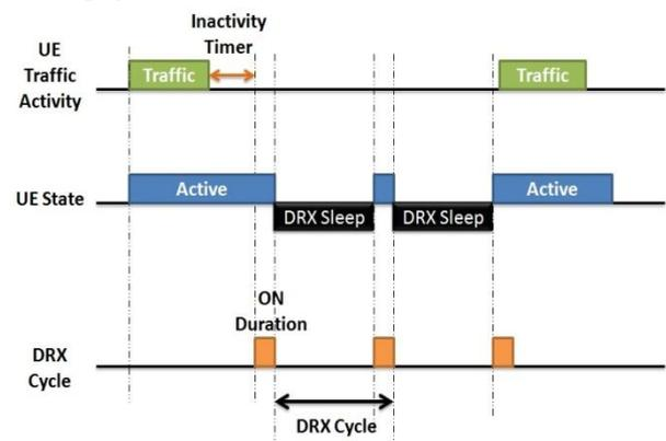
Fig. 1: UE state based on DRX cycle and Inactivity Timer in Idle state.
