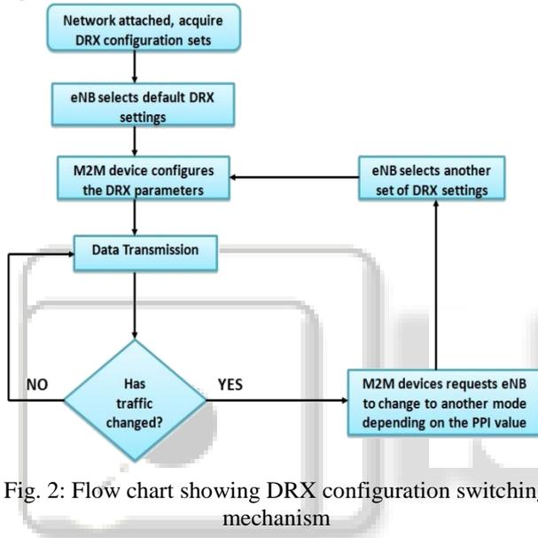
Fig. 2: Flow chart showing DRX configuration switching mechanism
