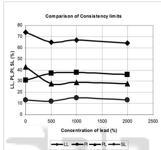
Fig. 2: Variation of index properties on addition of lead
