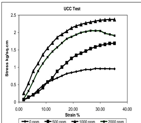
Fig. 1: Variation of strength on addition of lead
