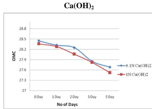
Fig.5.2: OMC vs. Number of days of pore fluid of Ca(OH)<sub>2</sub>
