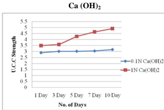
Fig.5.8: U.C.C Strength vs. Number of days of pore fluid of Ca(OH)<sub>2</sub>
