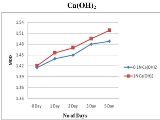
Fig.5.4: MDD vs. Number of days of pore fluid of Ca(OH)<sub>2</sub>
