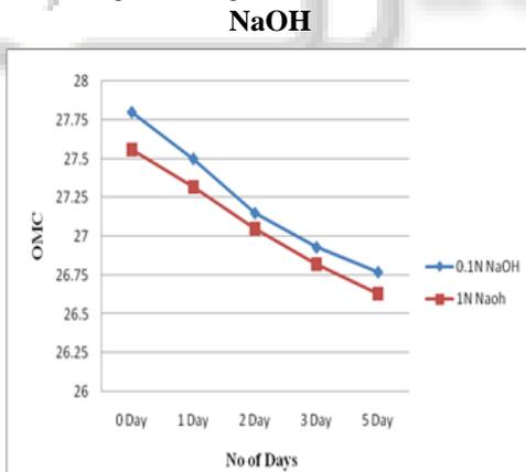
Fig.5.1: OMC vs. Number of days of pore fluid of NaOH
