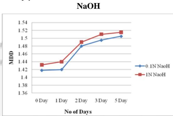
Fig.5.5: MDD vs. Number of days of pore fluid of NaOH
