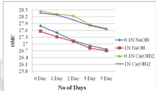
Fig.5.3: OMC vs. Number of days of both concentrations of pore fluids of Hydroxides
