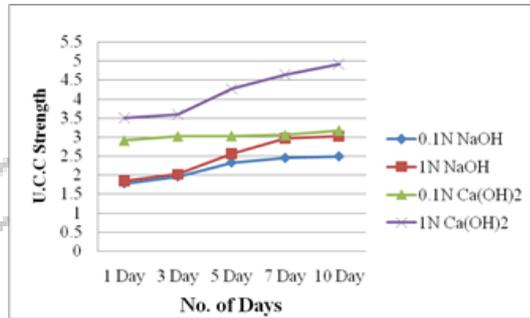
Fig.5.9: UCC Strength vs. Number of days of both concentrations of pore fluids of Hydroxides
