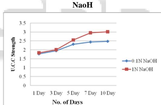
Fig.5.7: U.C.C Strength vs. Number of days of pore fluid of NaOH
