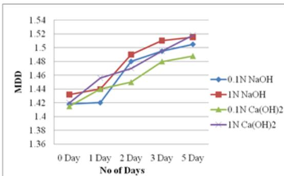
Fig.5.6: MDD vs. Number of days of both Concentration of pore fluids of Hydroxides
