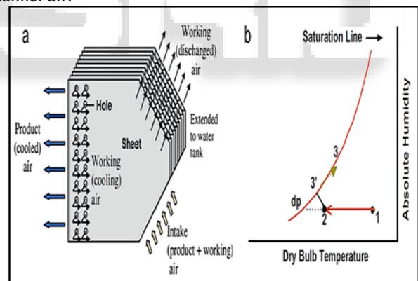
Fig. 5: Structure and operation of the M-cycle counter-flow heat exchanger for indirect evaporative cooling. (a) Structure illustration and (b) air treatment process—psychrometric [1]
