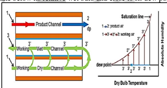
Fig. 3: Principle of the heat and mass exchanger based on M-cycle and its representation on psychrometric chart [1]
