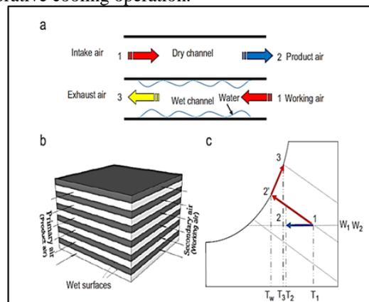
Fig. 2: Conventional IEC heat and mass exchanger. (a) Working principle of the indirect evaporative cooling, (b) Configuration of the type IEC heat and mass exchanger and (c) Psychrometric illustration of the air treatment process in the IEC heat and mass exchanger [1]
