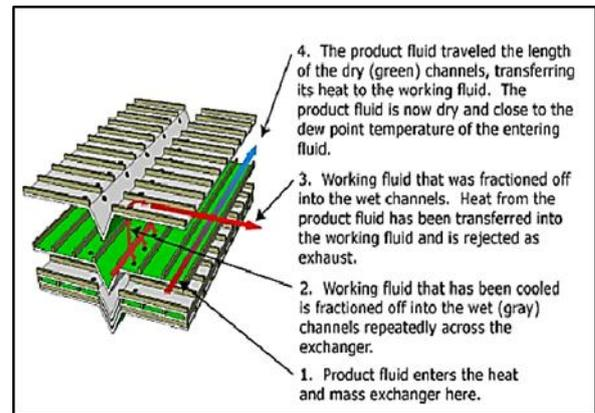
Fig. 4: Schematic of a heat and mass exchange module based on M-cycle [19]
