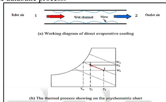
Fig. 1: Working diagram of (a) direct evaporative cooling and (b) thermal process showing on the psychrometric chart [19]
